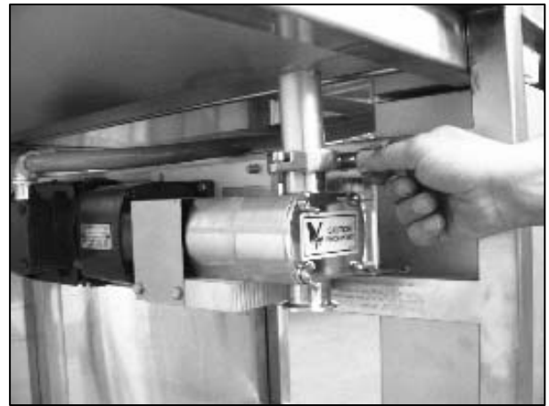
8. Install the upper clamp.
